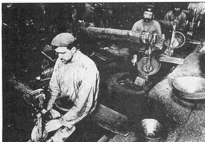
Brass pans being formed under battery hammers at Stolberg, Germany in 1905, an identical process to that operated at Chew Mill until the 1870's and at Saltford Mill until 1905. Photograph by courtesy of Dr. Karl Schleicher, Stolberg
